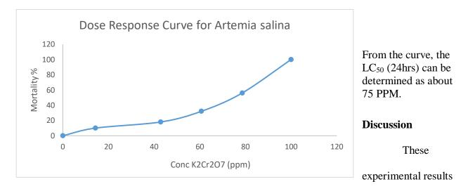
show that the mortality rate of Artemia salina increases with the increasing concentration of potassium dichromate (Ferraz Filha *et al.*, 2012). From the dose curve, the  $L_{50}$  of the larvae seem to be about 75 ppm.
